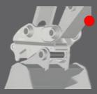
Unlock safety knuckle with the switch - buzzer is sounding at 2 beeps a second as the safety knuckle is retracted.
