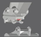
After 5 to 10 seconds the safety knuckle re-engages to the safe position.
