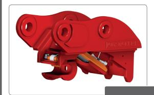
Though as classified as a wedge style coupler meaning a mechanical lock is not required, the X-Lock features the redundant RearLock safety device that ensures the wedge does not retract in the case of hydraulic failure.
